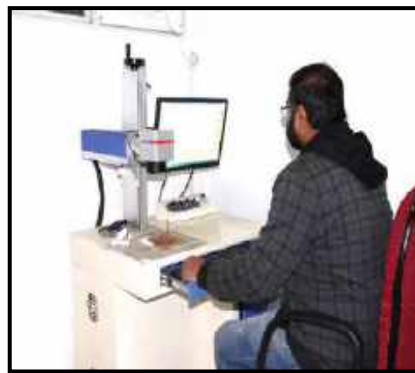
Fiber Laser PCB Milling Machine for the production of high-quality PCBs with fine features
